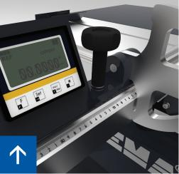
Electronic reader of the crosscut fence stopper with absolute memory function and 0.1 mm accuracy (optional).
